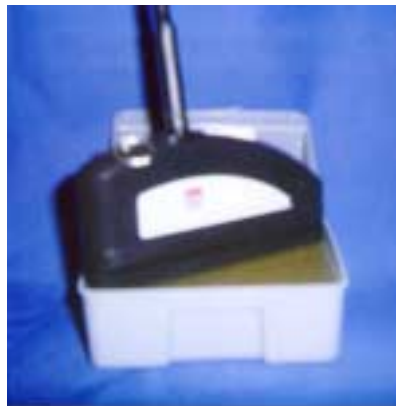
Figure 21 Probe placement in phantom for calibration of machine. Be sure probe is inserted so metal ring is to operator's left.
