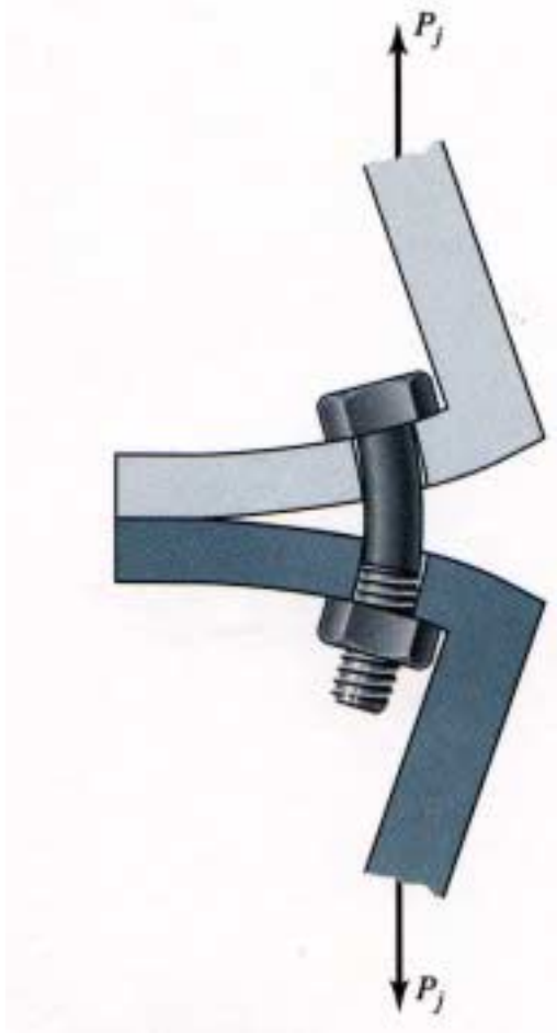
Exaggerated Deformation in Joint
