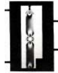
Photoelastic fringes in a narrow plate with hole loaded in tension.
