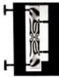
Photoelastic fringes in an notched beam loaded in bending.
